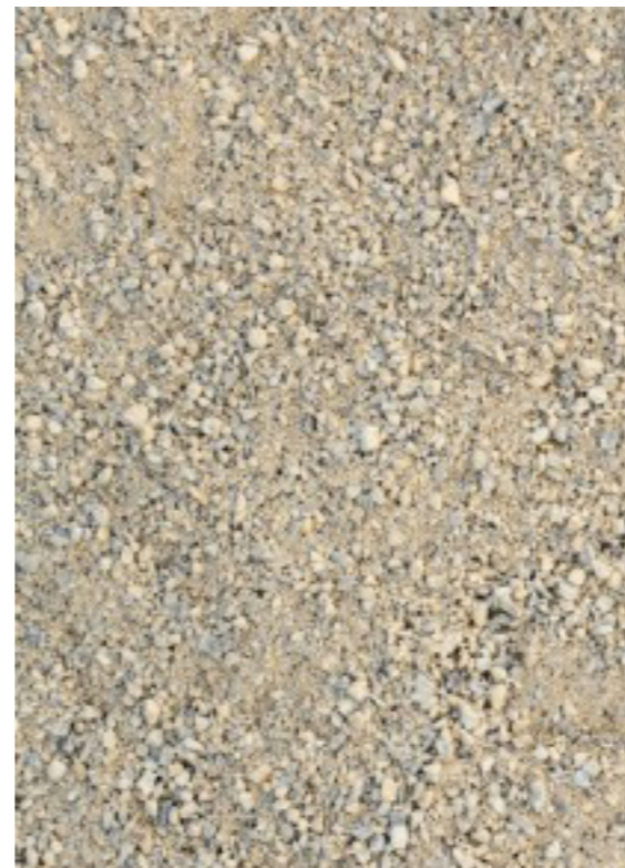
Gherang gravel path. Vehicle loaded sub-base
