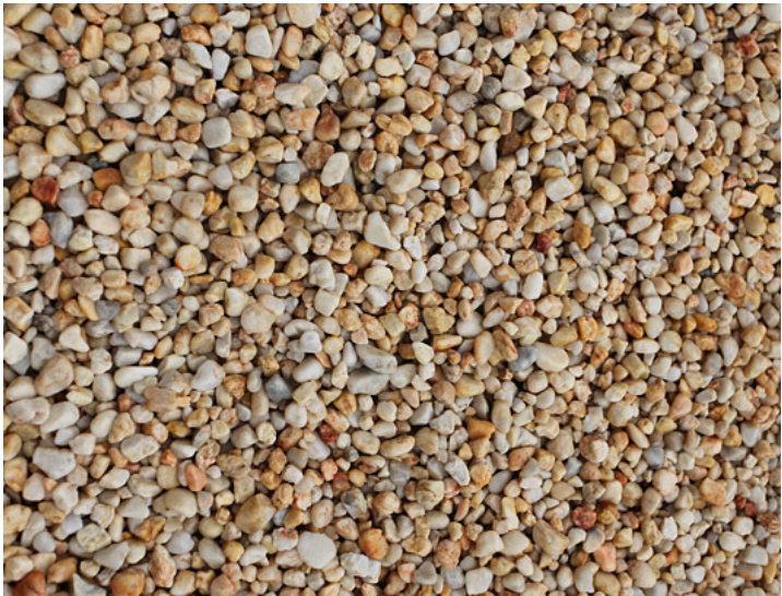
Porous materials such as gravel allows for onsite stormwater infiltration
