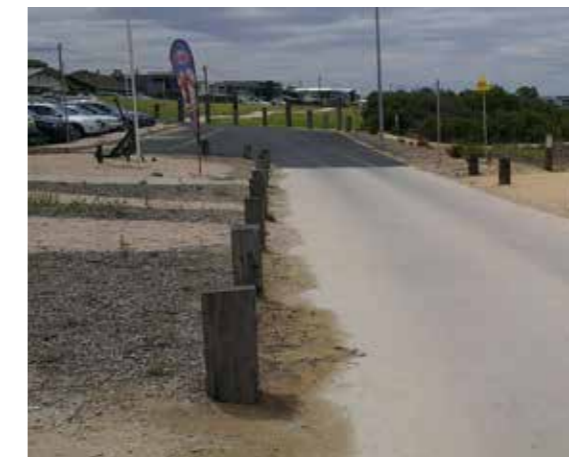
I.3 Change in paving material to indicate shared zone / areas
