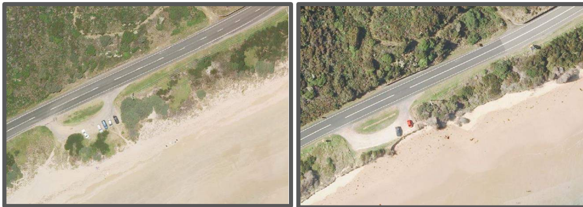
Image 8a: Eastern View car park in 2008 & b: 2011 showing approximately 15m of shoreline recession.
